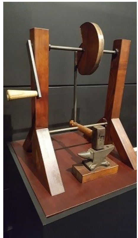
Model of a forging hammer designed by Leonardo, from “Da Vinci Live!” at the Science Museum of Virginia.
