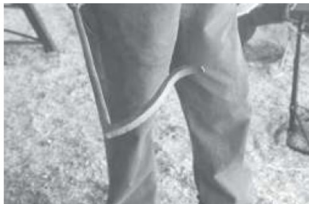
Finished hold fast. The curve in the arm was completed at the anvil.
