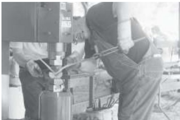
Bending the corner in a V block on the power hammer
